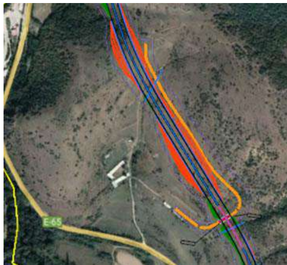
Figure 159 Alignment of the Motorway passing near the sheep pen at the location III (orange colour is a new road with underpass that can be used by sheep)
