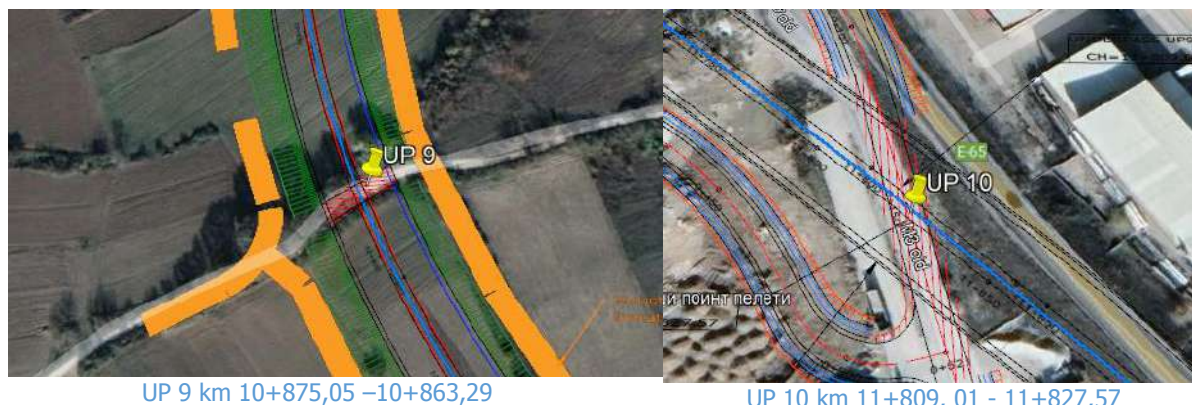
Figure 20 Under passes along the alignment
