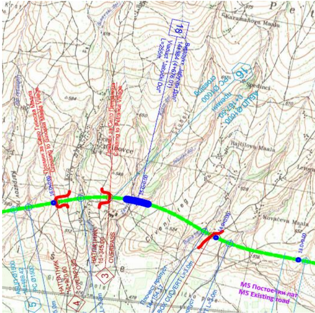
Figure 7 location of the viaduct 18
